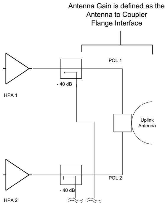
*Figure A.3-3. Uplink Antenna Gain Interface*
