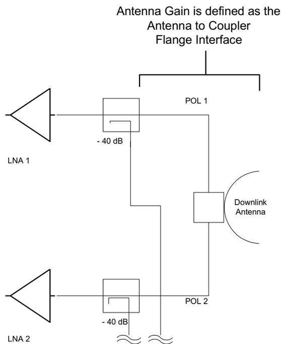
*Figure A.3-4. Downlink Antenna Gain Interface*
