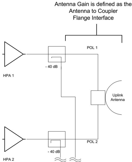
*Figure A.3-3. Uplink Antenna Gain Interface*
